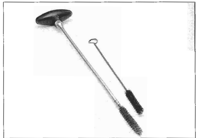
6.2a A selection of brushes is required for cleaning holes and passages in the engine components
