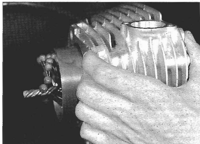
14.14 Move the hone rapidly up-and-down without stopping
