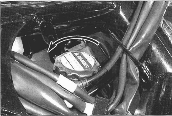
19.7 To remove the radiator cap, turn the cap counterclockwise to the first stop, let any residual pressure escape, then turn the cap counterclockwise until it's free
