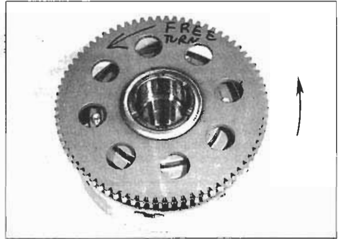
32.4b Hold the rotor and turn the gear; it should turn freely counterclockwise, but lock up when you try to turn it clockwise
