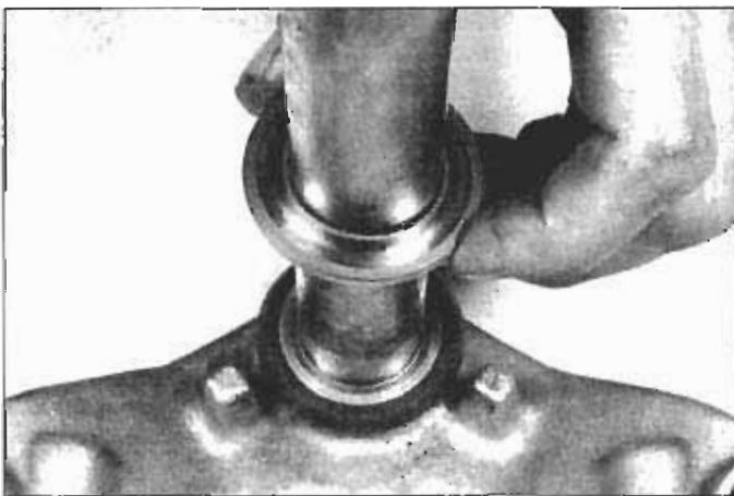
6.18b . . . then install the lower bearing inner race with its bearing surface facing up, and press the race onto the stem with a section of pipe (taped to protect the bearing surface)
