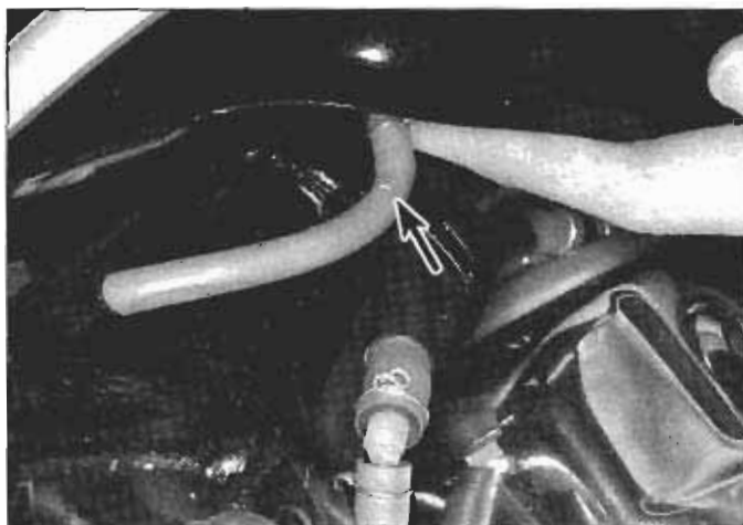
2.27b On California models, detach the breather hose from the right side of the tank
