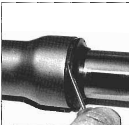
5.6 Pry the dust seal out of the fork slider with a small screwdriver and slide it out of the way; don't slide the seal over rough spots if you plan to reuse it
