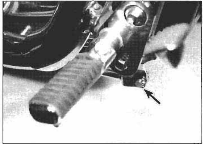
9.4a Remove the cotter pin, pull out the clevis pin (arrow) and disconnect the middle brake rod from the brake pedal arm . . .
