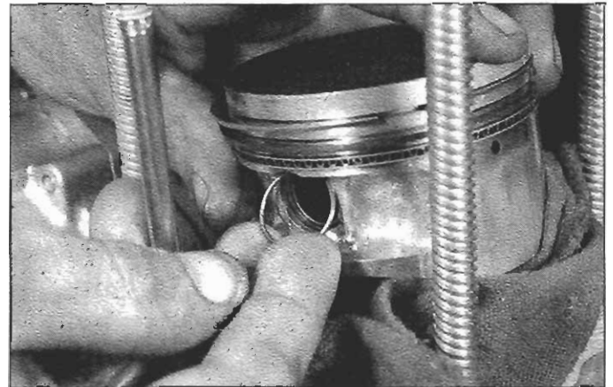
15.18a Slip the circlip into its bore with its gap away from the piston cutout . . .
