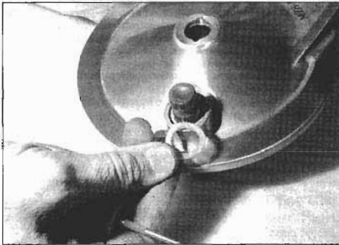
8.6c Remove the felt seal from the brake cam spindle
