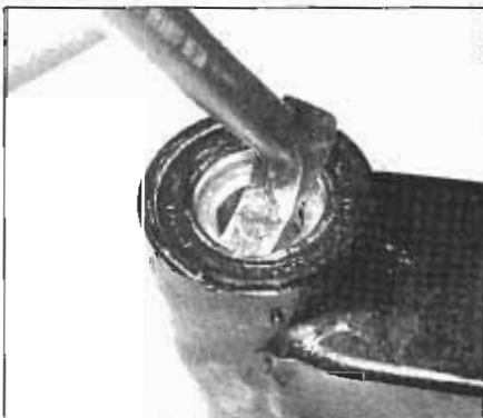
11.3a Pry out the old grease seals from the swingarm with a seal removal tool or screwdriver
