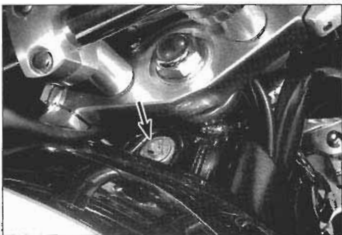
2.25 Remove the front fuel tank mounting bolt (arrow) and collar; replace the rubber insulator if it's damaged
