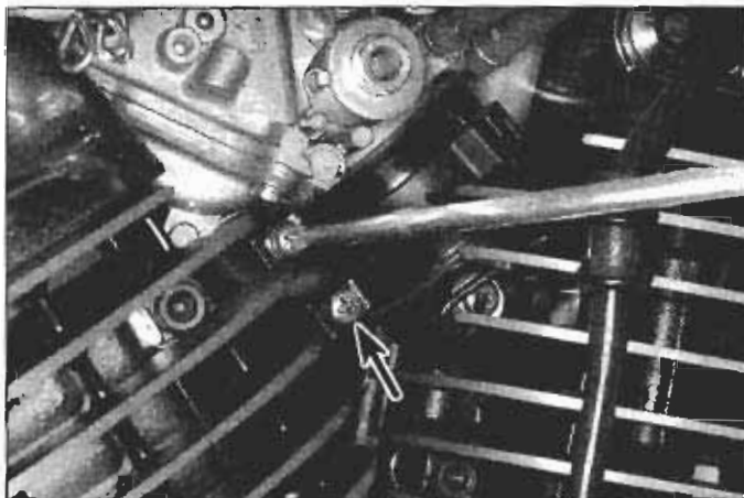
12.12a Loosen both insulator clamp screws ...
