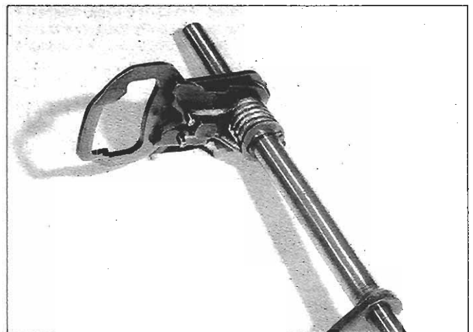
22.24a Before installing the right gearshift spindle, make sure that the ends of the return spring are positioned on either side of this lug, as shown
