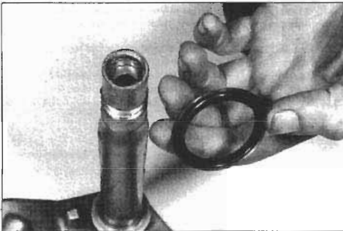
6.18a Install a new seal with its concave side down . . .
