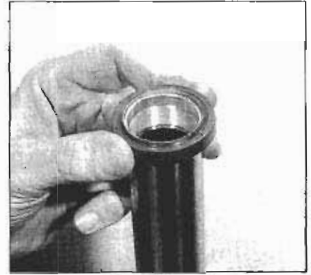
5.25b . . . and install the seal on the fork tube; don't let the upper edge of the fork tube damage the seal lip
