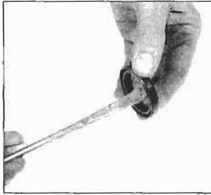
5.25a Coat the inner lip and the outer circumference of the new seal with grease or fork oil . . .
