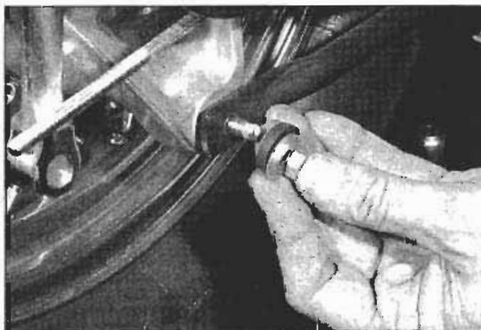
8.3b . . . remove the nut and the metal and rubber washers from the bolt, slide off the stopper arm and remove the bolt from the brake panel
