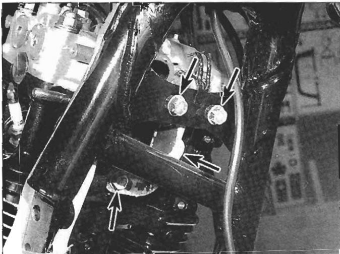
5.25a Remove these two upper mounting bolts (arrows) ...
