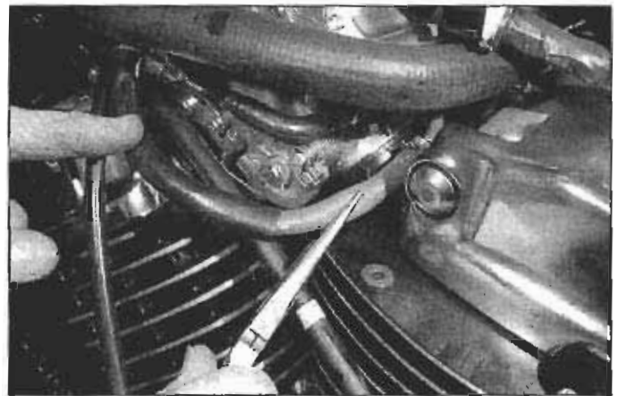
12.11c ... and detach the EVAP hose from the left (rear cylinder) carburetor
