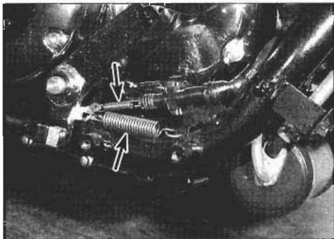
9.18a After removing the footpeg bracket, disconnect the pedal return spring and the brake light switch return spring (arrows) . . .
