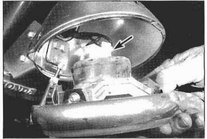
7.2 Tilt the cover out of the headlight assembly and disconnect the wiring connector
