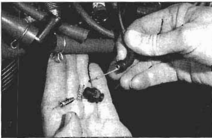
12.10b ... and separate the SE valve, spring and locknut from each cable
