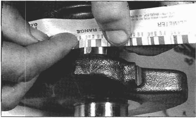
27.15 Place the Plastigage scale next to the flattened Plastigage to measure the bearing clearance
