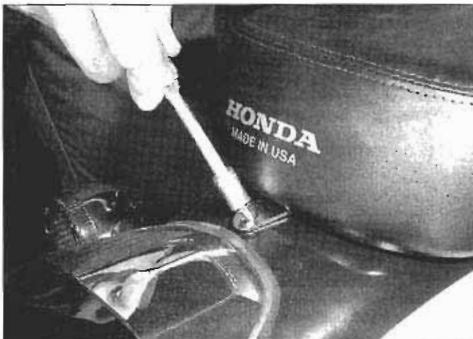
6.3a To detach the seat on VT1100C2 and VT1100T models, remove this cap nut . . .
