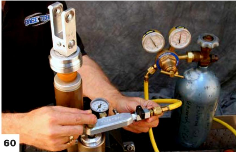
Fill up with nitrogen using the Pro Shock Nitrogen Gauge.
