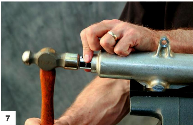
If the compression bolt is stuck, hammer on the compression bolt with a properly sized socket to help break the thread loose. Again, if you do this be aware you can damage both the socket and the bolt. Wear safety glasses.
