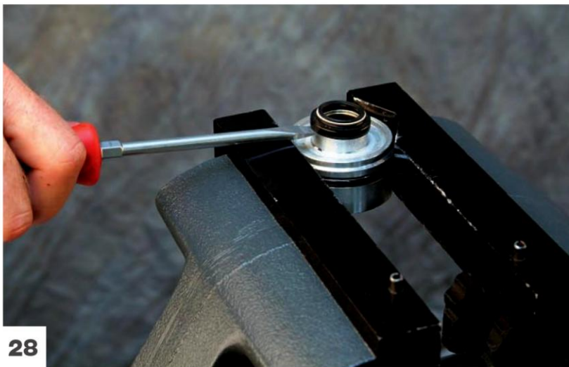
Remove the dust seal. Note the notch in the vise jaws. If you hold the seal head with the top surface below the top of the vise jaws, you can pry on the edge of the jaws.
