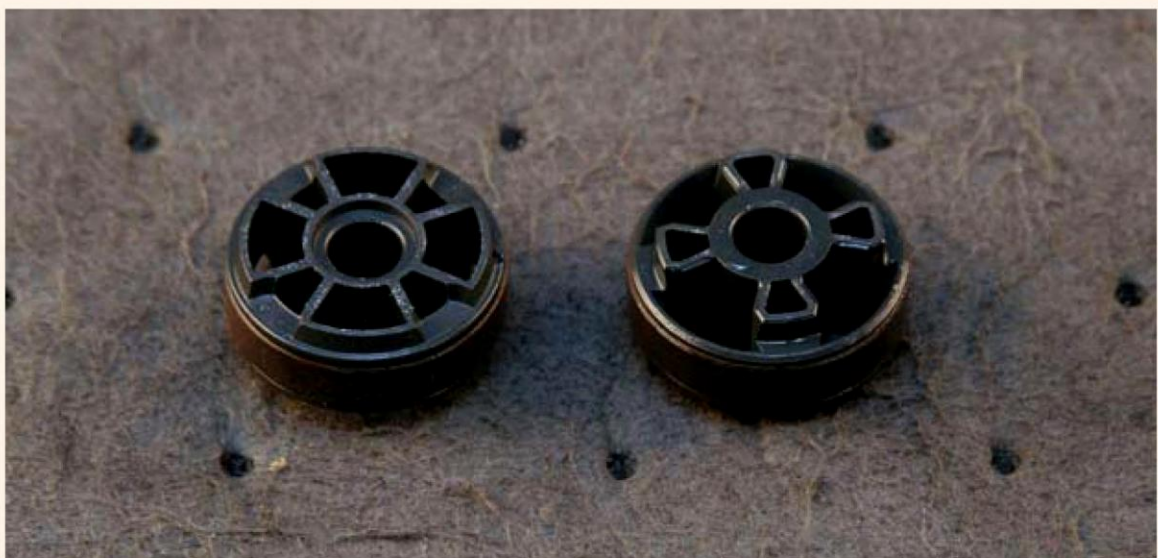
Every valve has two distinct sides. The piston on the left is showing the recessed side. This is the mid-valve/check valve side. The piston on the right is showing the flat side, which is the rebound valving side.
