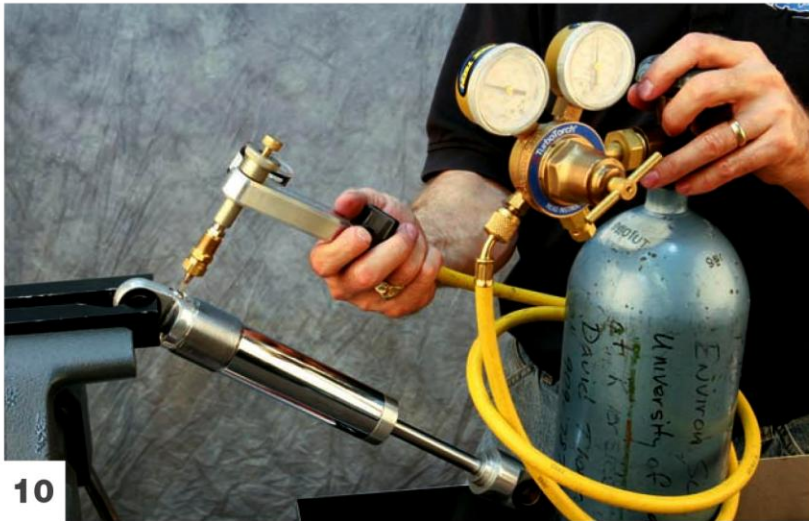
Pressurize the shock with the nitrogen needle.
