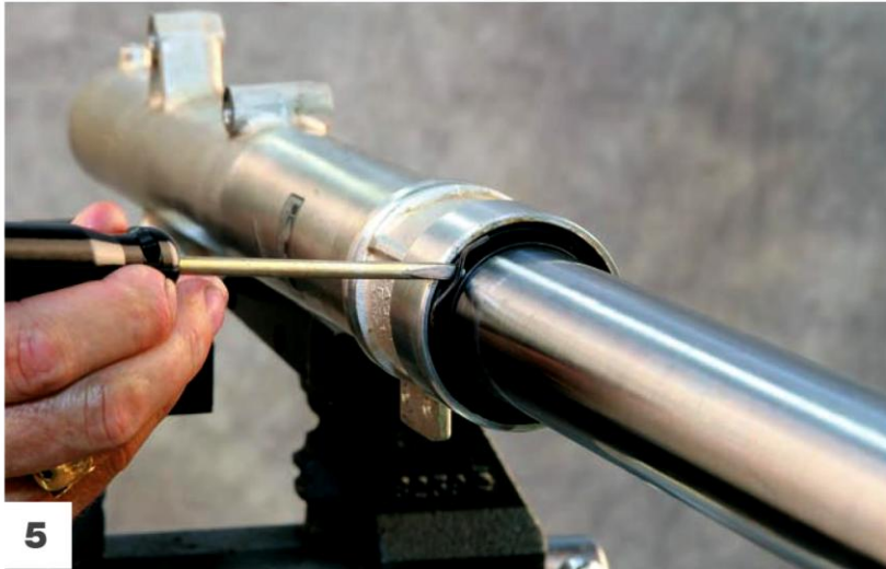
Remove the seal clip with a clip tool or small screwdriver.
