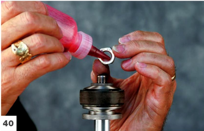
Use Loctite on the shaft nut.
