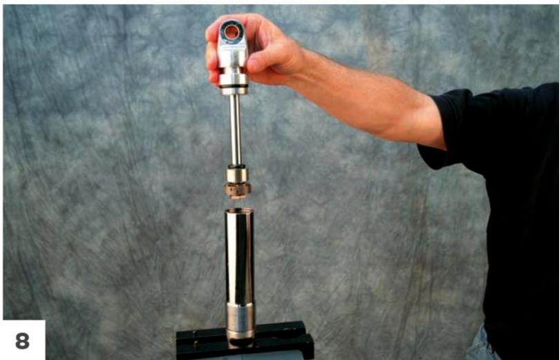
Insert the shaft assembly into the shock body.
