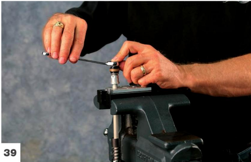
Remove the rebound nut.
