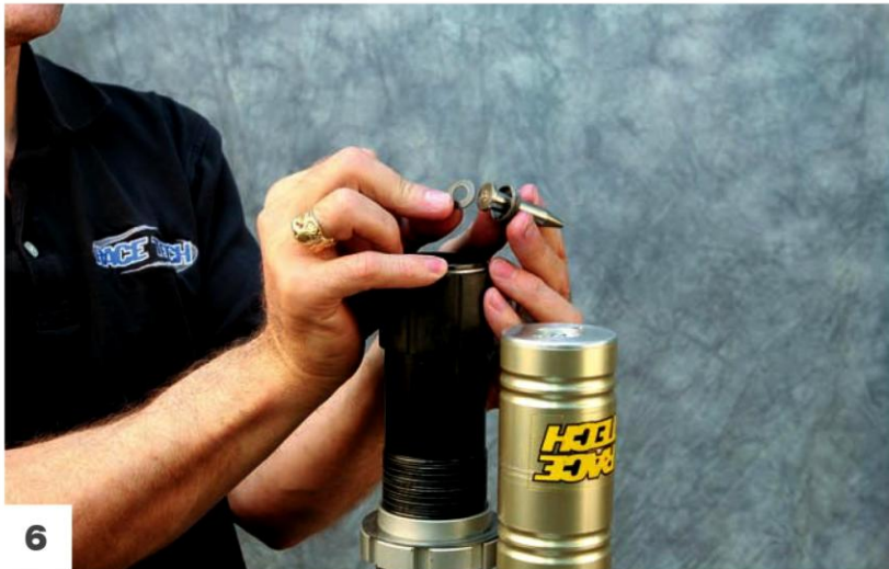
This is the stock metering needle assembly.
