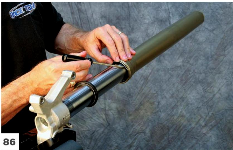
Seat the clip in the groove with the clip tool or a small screwdriver.
