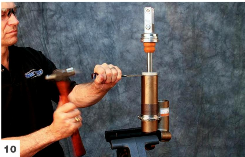
Remove the shock body cap with a sharp wood chisel. Some models screw on, so don't get too excited with the chisel unless you are sure. Note: Most Showa, KYBs, and Öhlins are pressed on. Penske, Works Performance, and early Öhlins are screwed on.
