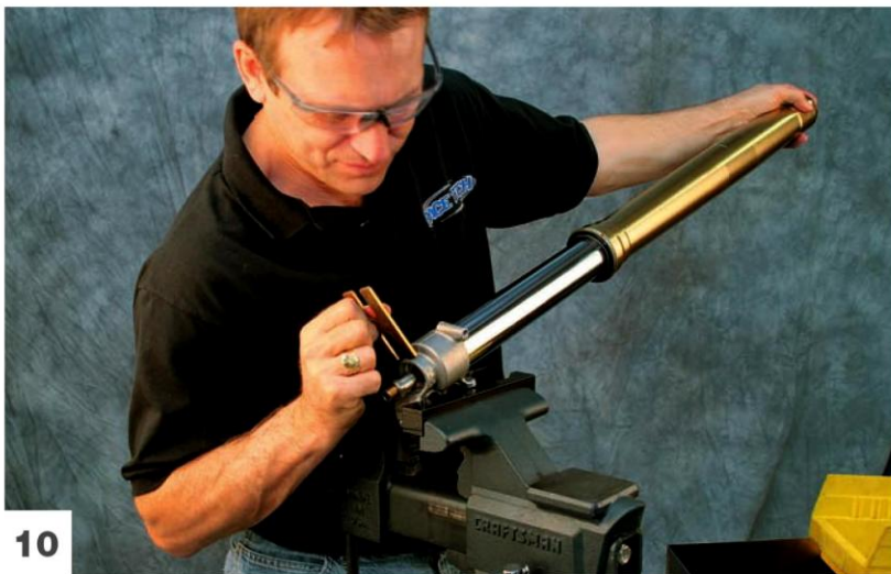
Compress the fork and remove the clip tool.
