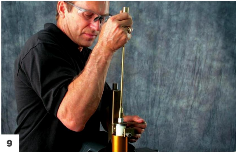
Thread on the bleeding tool, pull up, and remove the clip.
