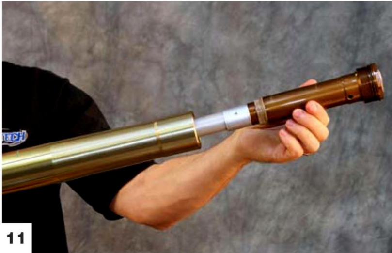
Remove the cartridge.
