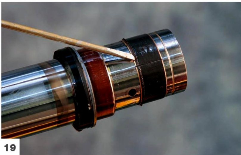
Some forks may suffer damage to the Teflon bushings during disassembly (as shown). This is common on 46mm KYBs. It's good to have extra bushings on hand.
