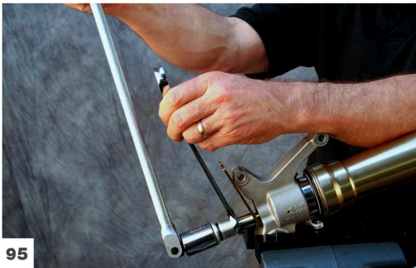
Tighten the jam nut.
