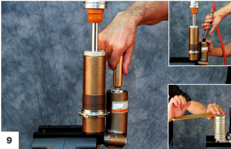
Remove the reservoir cap with the Race Tech Reservoir Cap Removal Tool. Make sure the tool is screwed on all the way. (Alternatively you could use compressed air to blow the cap off.) For WP shocks with a threaded cap, use a pin spanner.
