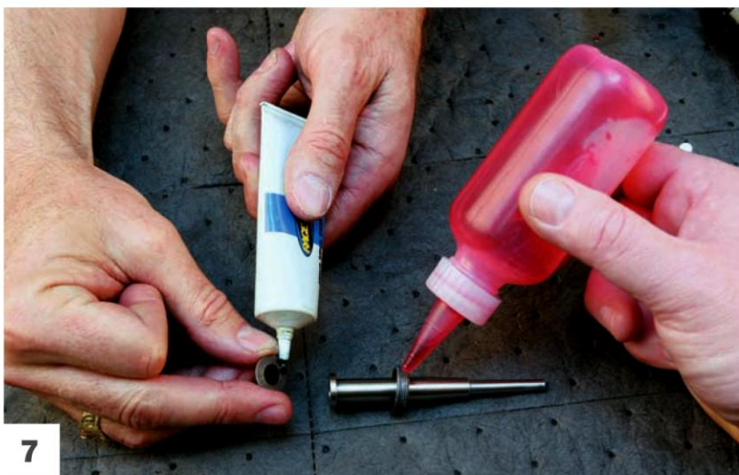
This is the Race Tech Telescopic Needle. Apply thread locking compound on the retaining collar and a small amount of Race Tech Ultra Slick Grease on the Bellville washer during installation. The grease temporarily sticks the washer to the end of the needle.
