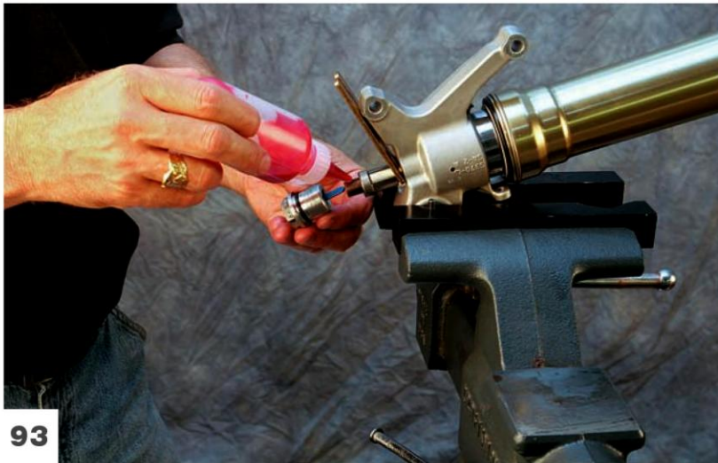
Put a drop of Loctite on the damping rod thread.
