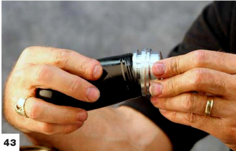
Reinstall the valve core and bladder onto the reservoir cap.
