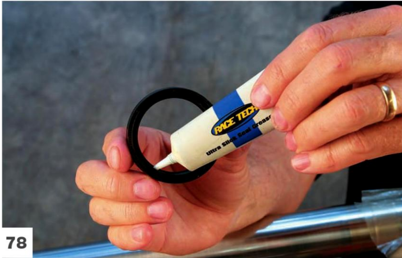
Grease the fork seal and wiper.
