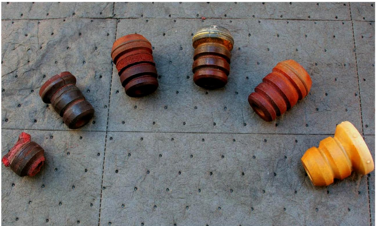
Note: A bottom-out bumper is a consumable item—only the one on the right is still usable. Always inspect your bumper and replace it if necessary.
