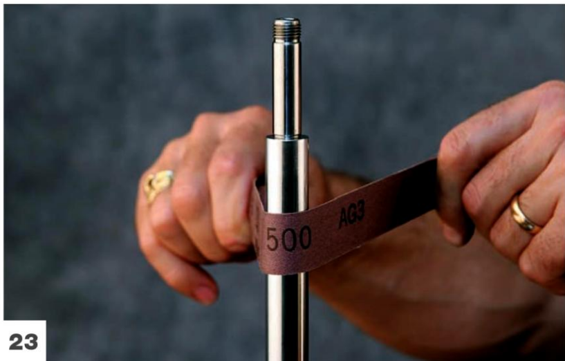
Polish the shaft with 500- or 600-grit sandpaper.
