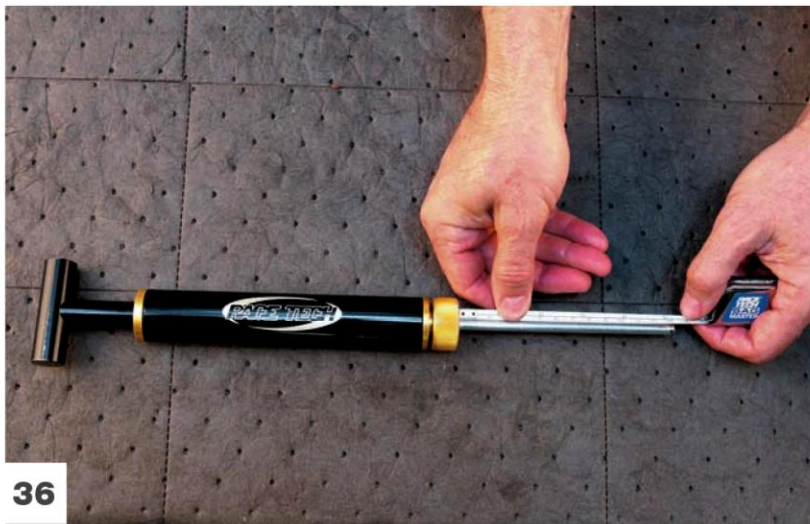
Adjust the tube extension on the oil sucker tool to equal the dimension of the target oil level.
