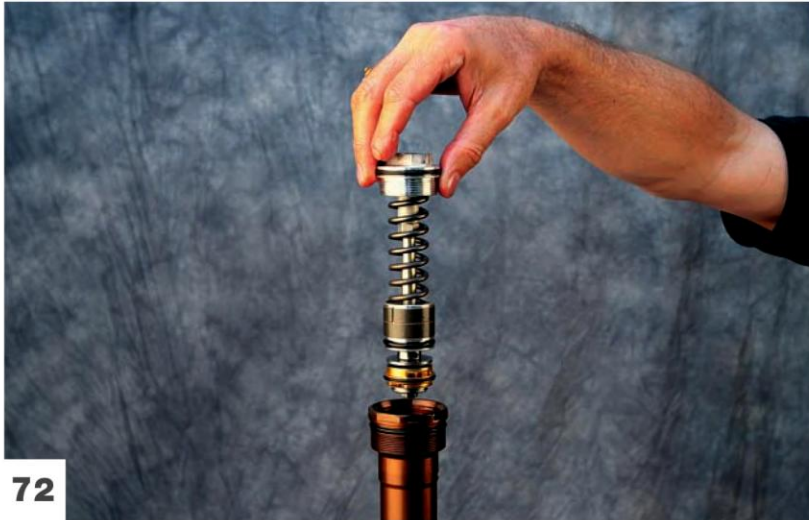
Insert the compression valve assembly.
