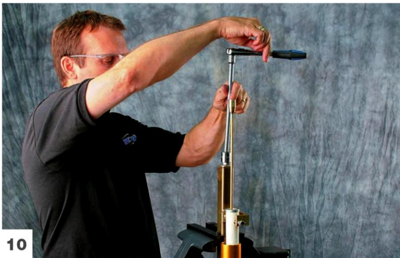
Release the preload.
