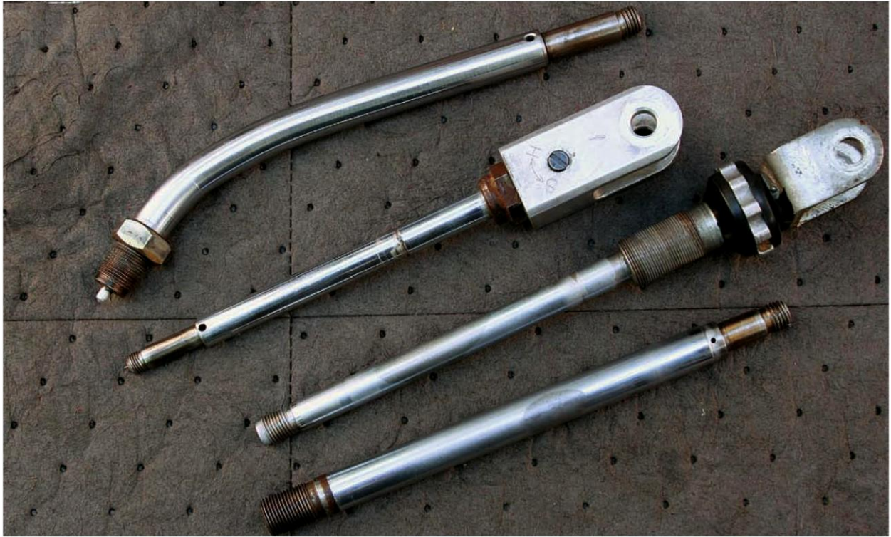
Behold the Shock Shaft Hall of Shame. From top to bottom: Bent shaft caused by ramming after linkage bolt came out; vise grips are not for holding the shaft end; and two examples of worn-through hard chrome from extreme use. Hint: don't take off shock mud flaps.
