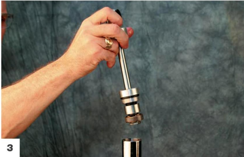
Remove the shaft assembly.
