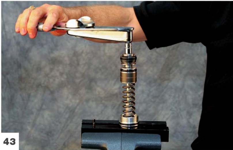
Torque the compression valving shaft nut. (stock/G2-R)
