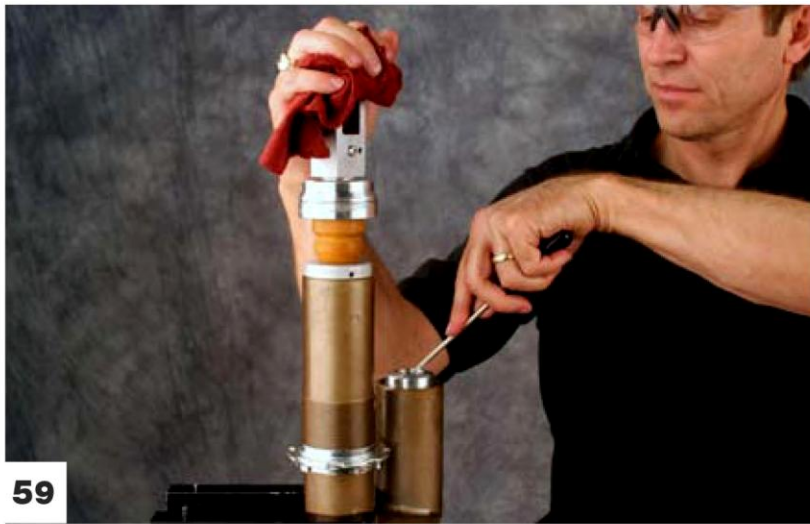
Compress the shock while depressurizing the bladder.
