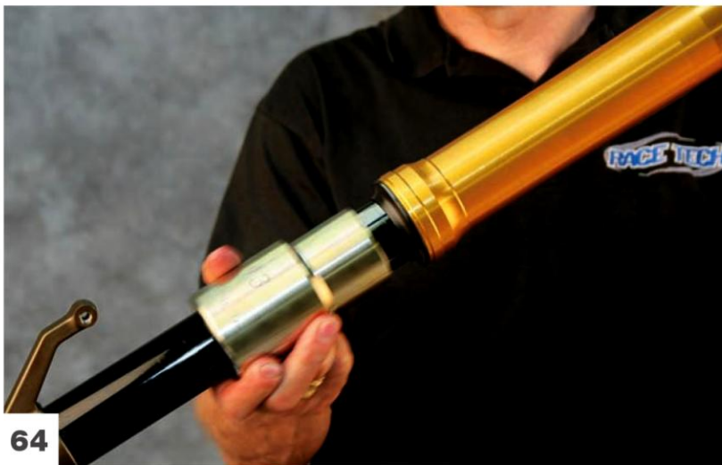
Install the wiper with the seal driver.
