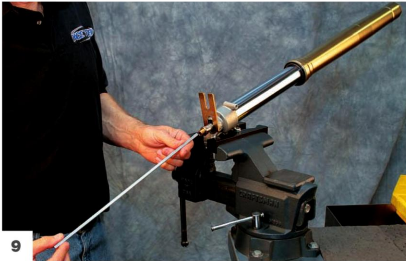
Remove the D-shaped rebound adjuster rod.
