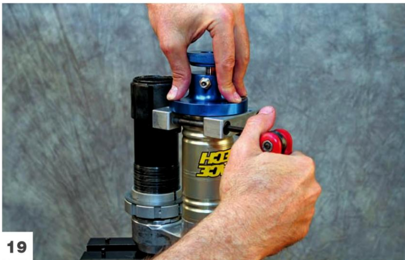
With the Allen bolt loosely installed, attach the Race Tech WP Nitrogen Charging Tool. Push down on the tool as you tighten the holding clamp.
