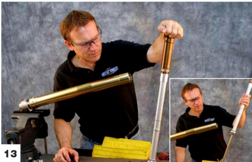
Check for evidence of good seals. Compress the cartridge all the way, and it should return to the fully extended position by itself. If it doesn't, the internal oil level may be low, possibly caused by leaking shaft or reservoir seals. If it is a 05 YZ, it will not return all the way as the pressure spring is too short from the factory. Also it may not extend all the way if there is only slightly too much friction.
