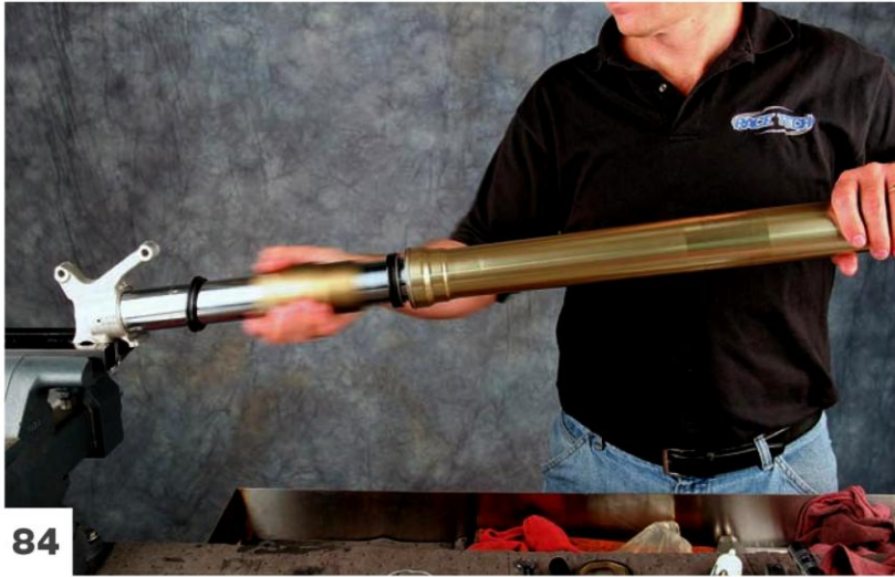
Install the oil seal with the seal driver.
