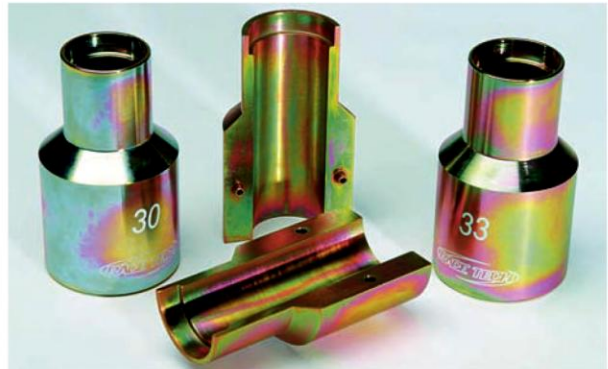
Series Seal drivers: Split design for both conventional and upside-down forks.
