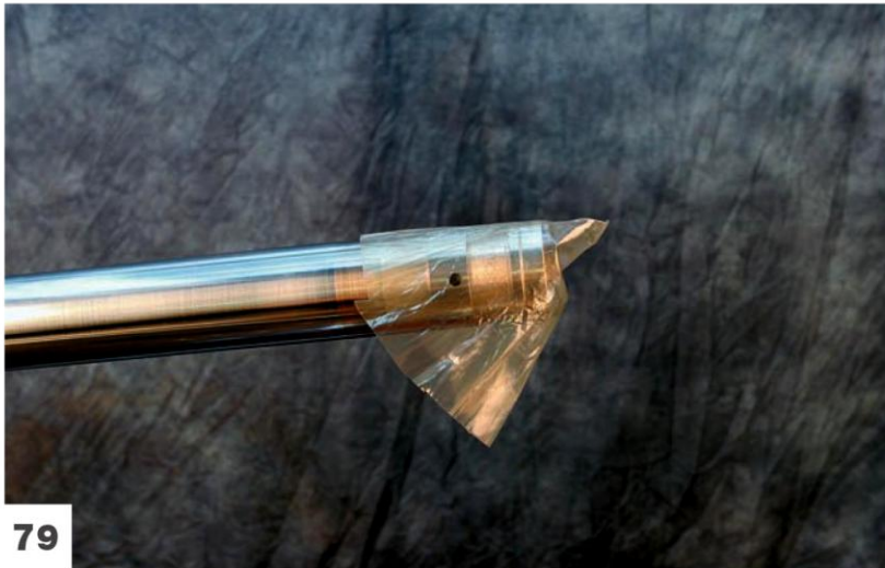
Use the corner of a heavy gauge plastic bag and place it on the end of the fork tube. This will protect the seal from the sharp edges of the inner bushing groove.
