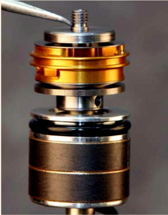
Incorrect stack height on a G2-R
