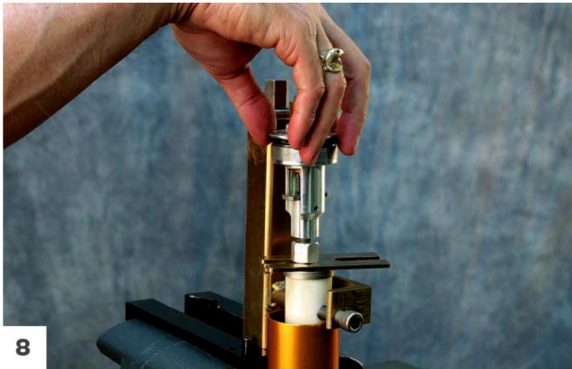
Remove the fork cap.
