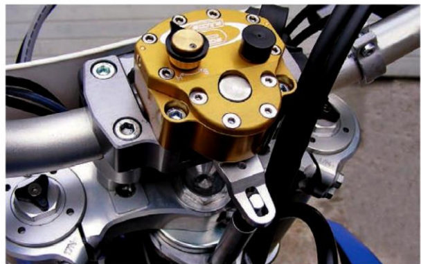
This Scott's Steering Damper is a rotary vane damper that does an excellent job of controlling headshake. Even if headshake is not a problem, the damper allows the rider to relax quite a bit more.
