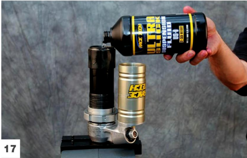
Fill the shock body with oil to a height of 40mm (1½").
