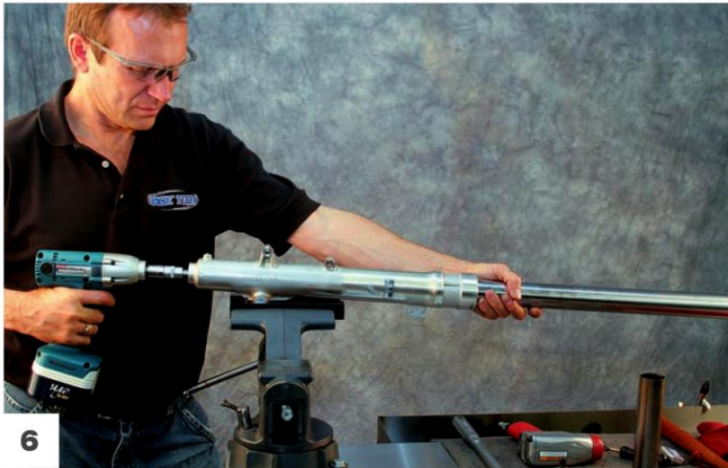
Loosen the compression bolt with an impact driver while pulling on the upper fork leg to keep it from spinning. If it continues to spin, you can reinstall the fork spring, spacer, and cap, then compress the fork. If it still continues to spin, you may have to make a holding tool for the damping rod.
