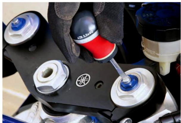
Most cartridge forks have the rebound damping adjuster on the fork cap. It will often be labeled with the letters "Ten" (tension) or "REB" (rebound). A few models, such as the 2009 Yamaha R1s, FZ1s, and many Moto Guzzis, have one fork cap for compression and the other for rebound.
