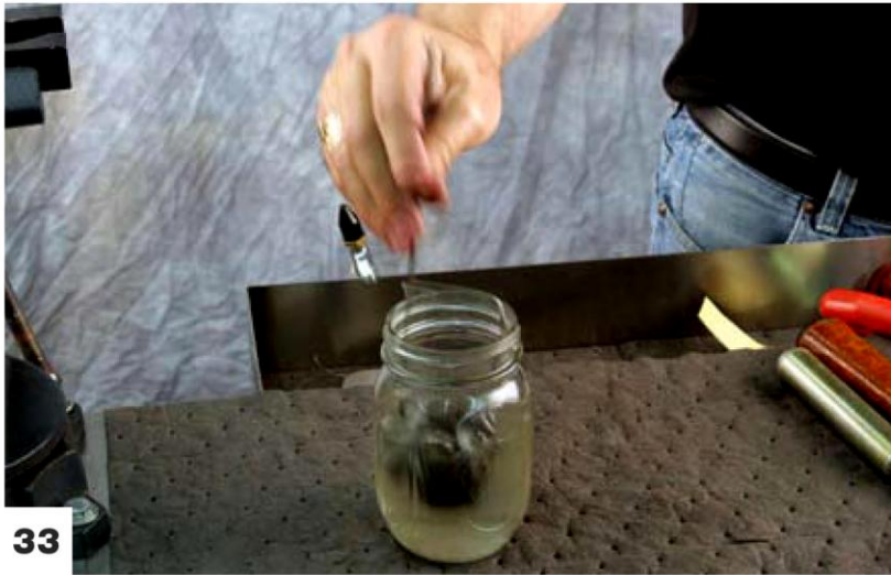
Clean the valving assembly in contact cleaner.
