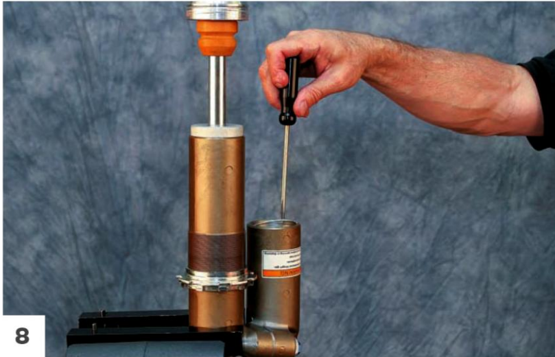
Remove the reservoir clip with the clip tool.
