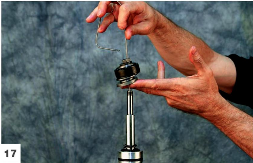
Remove the valving stack.
