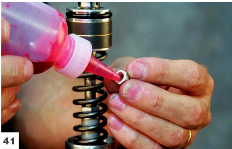
Apply a small drop of Loctite to the compression valving shaft nut.
