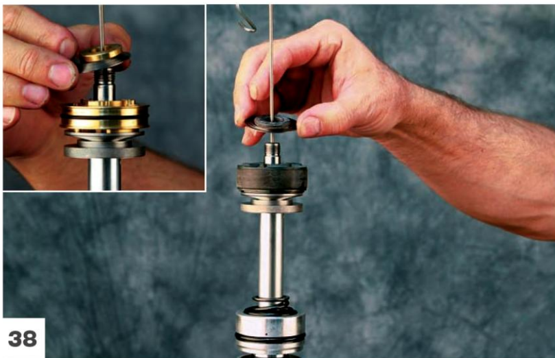
Install the piston and rebound valving. Use a Race Tech Gold Valve (inset) for improved damping action and tunability.
