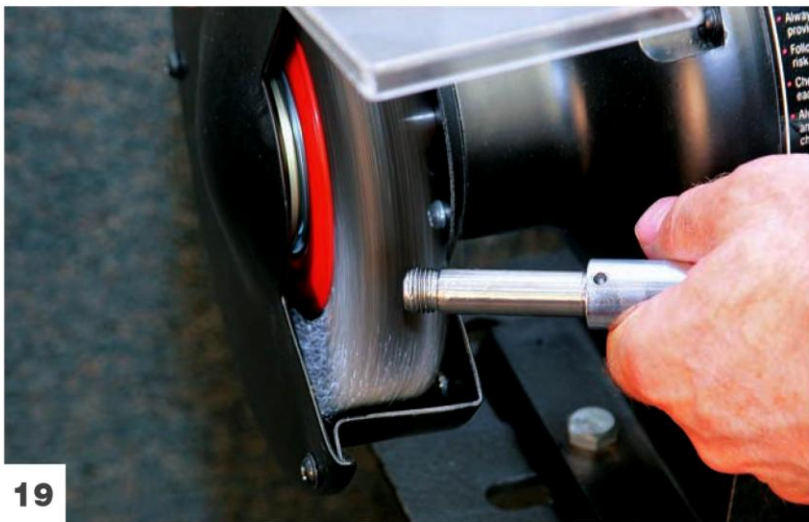
Wire wheel the end of shaft.
