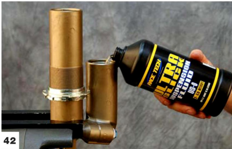
Pour Race Tech Ultra Slick Suspension Fluid into the reservoir first.
