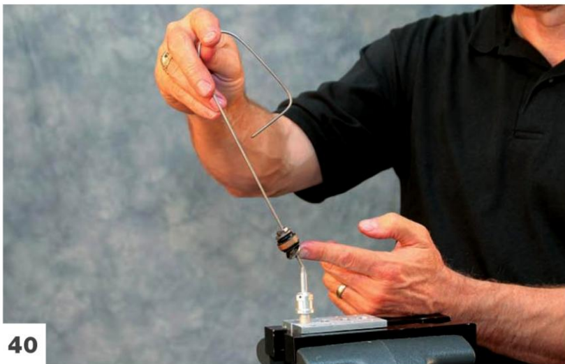
Remove the rebound valving.
