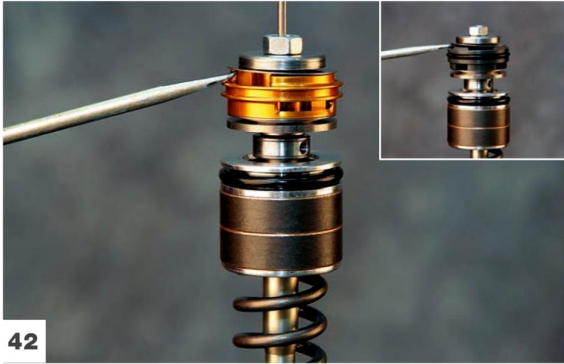
Check to make sure the check valve is free.
