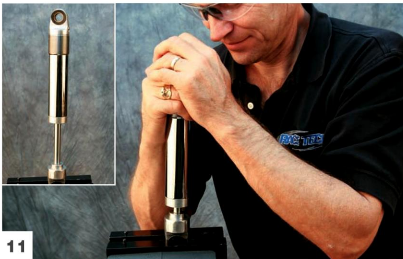
Compress and make sure the shaft extends completely. Note: Make sure emulsion shocks are mounted body up.
