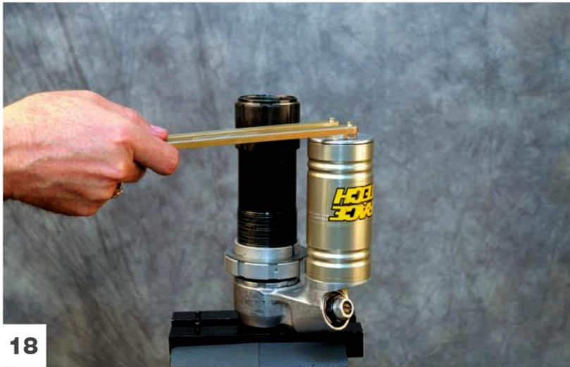
Lightly grease the O-ring and install the reservoir cap.
