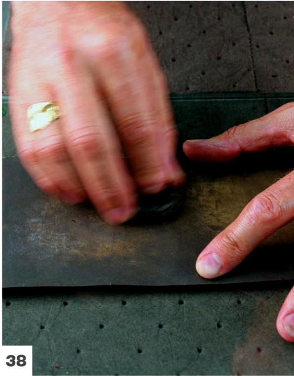
Surface the piston on 320-grit or finer sandpaper on a piece of plate glass.
