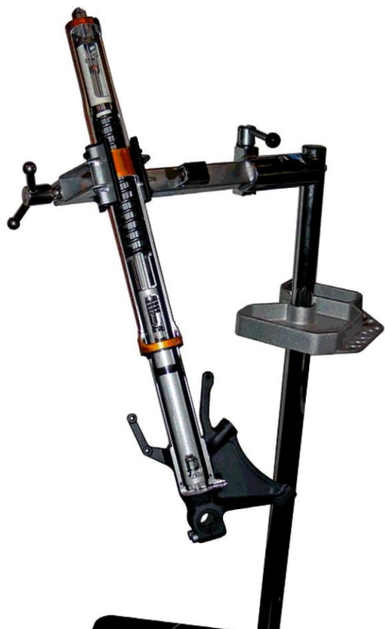
This Park Tool Vise was originally made for working on bicycles but can be used on forks as well. A bench-mount base is available for a bit more stability.
