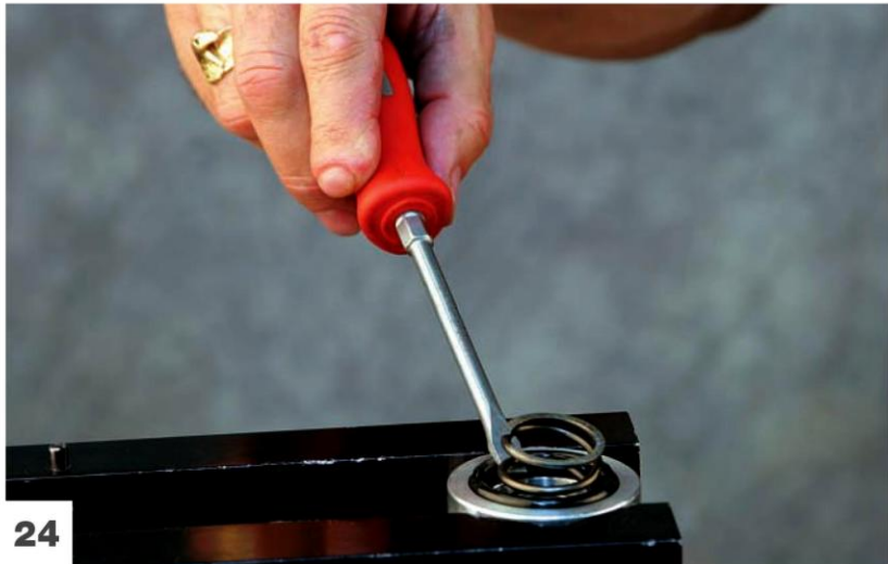
If the seal is being replaced, begin by removing the top-out spring from the seal head (for shocks that have one.)
