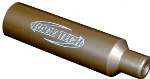
A reservoir cap removal tool screws onto the Schrader valve to facilitate removal of the bladder cap.
