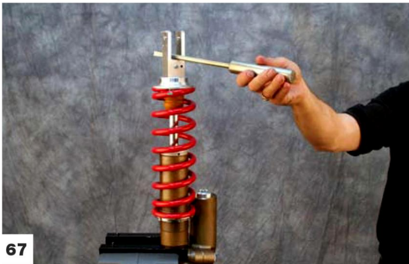
Line up the eyelets top to bottom. Make sure the adjusters are aligned correctly. Usually compression and rebound are on the same side but not always. Sometimes the shaft clevis has cutouts for linkage clearance. This is important.
