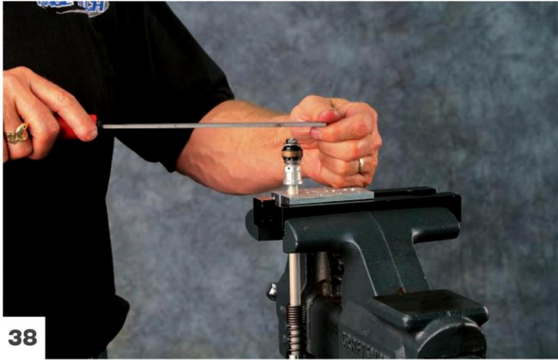
File the peening on the rebound valve.
