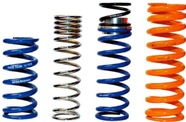
From left to right: straight-rate, single spring dual-rate, stacked dual-rate, and true progressive rate springs.
