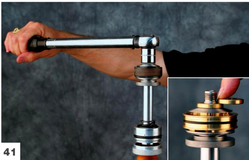
Check for proper stack height with the shaft nut and add an additional spacer (inset) if needed. Torque the shaft nut. The rebound base plate should cover the step at the end of the thread. The nut must have full engagement and not run out of thread onto the straight shaft.
