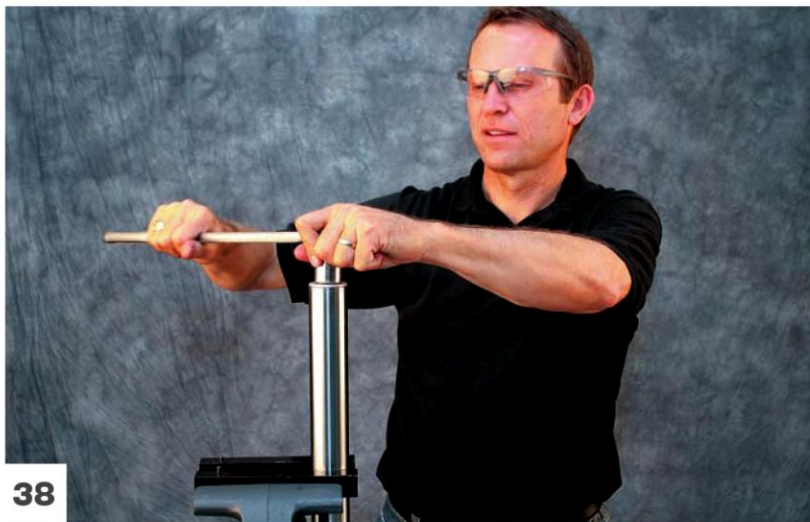
Install the fork cap and use a torque wrench to tighten it to manufacturer's specs.
