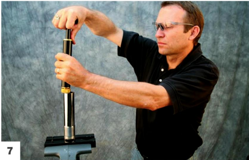
Set the oil level. This is critical as there must be more air space than the volume the shock shaft displaces (see Figure 3.34).
