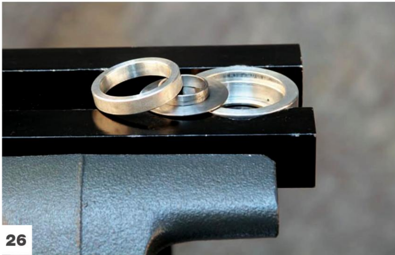
Remove the top-out bumper. Note: Some models do not have these pieces.
