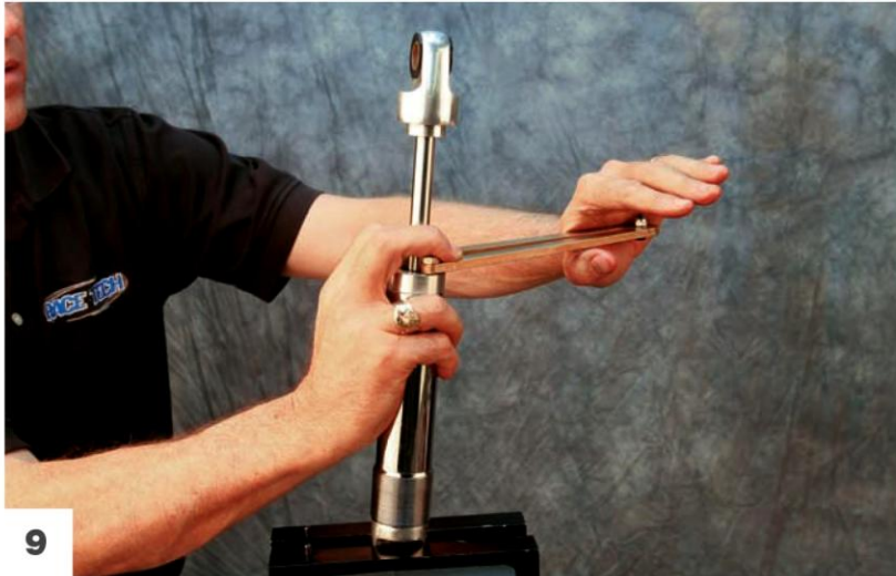
Tighten the seal head with Race Tech Pin Spanner.
