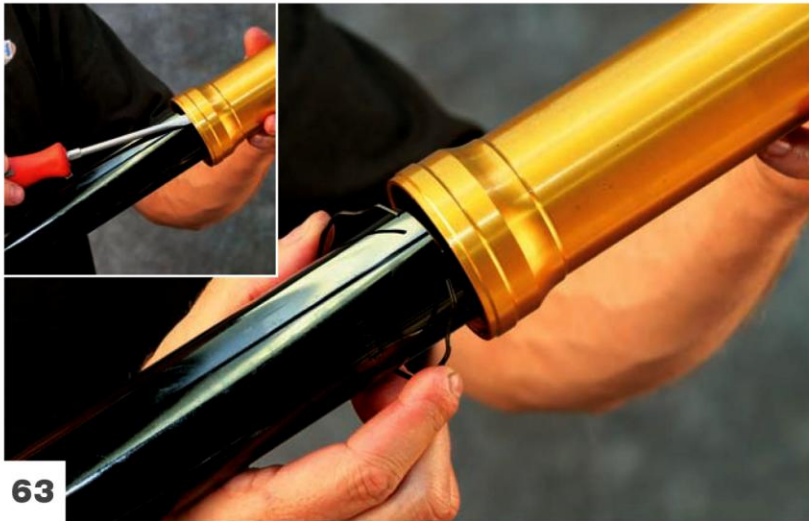
Install the seal clip and then seat the seal clip with a screwdriver.
