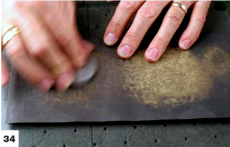
Surface the base plate on 220–280-grit sandpaper on a piece of plate glass.
