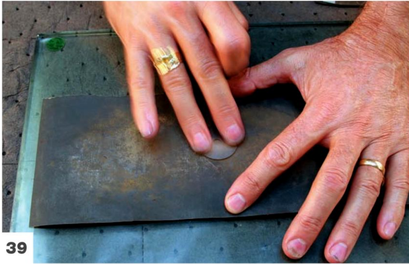
Surface the base plate.
