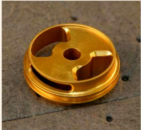
G2-R piston showing refill ports on the side and the recess on the compression face for creating preload and restriction.
