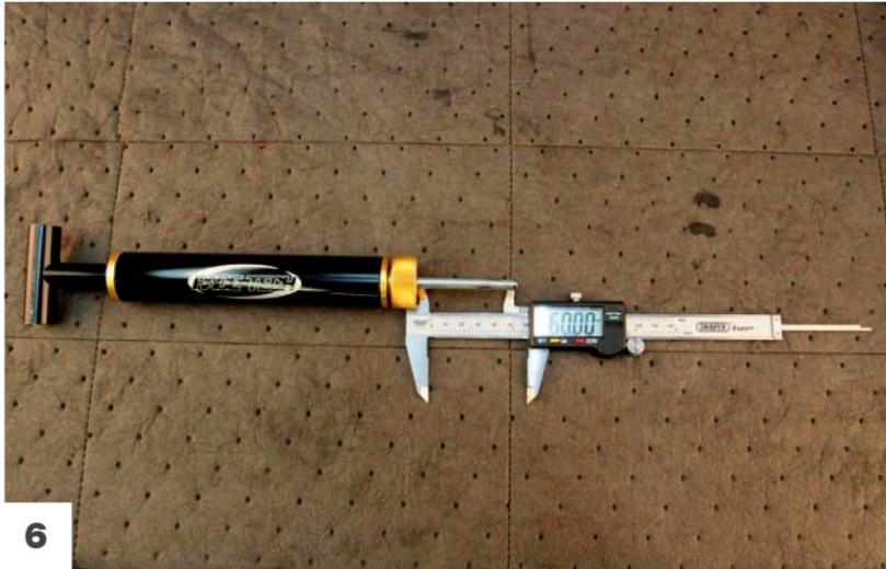
Adjust the tube extension on the Race Tech Pro Fork Oil Level Tool to the required oil level.
