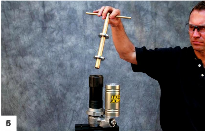
If charging the telescopic needle, use one of the RT TSST Series tools. There are three sizes.
