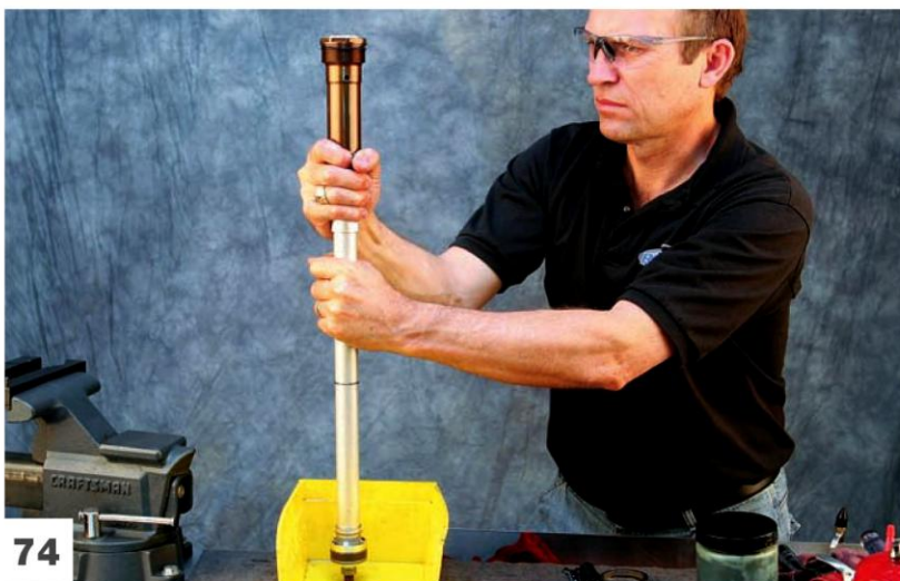
Set oil volume by compressing the cartridge all the way. The reservoir piston will move up until the piston no longer seals on the shaft where the "necked-down" portion of the shaft is. This is called the "assembly groove" on figure 3.32. Extra oil will go past the reservoir piston.
