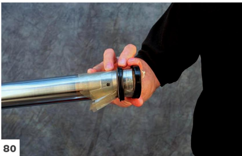
Slide on seal and wiper over plastic bag. Pulling the bag taut will further smooth the sharp edges, preventing damage. The seal and wiper are directional, so make sure they are on the right way with the dual-lipped part of the seal facing away from the fork bottom and toward the outer fork tube.
