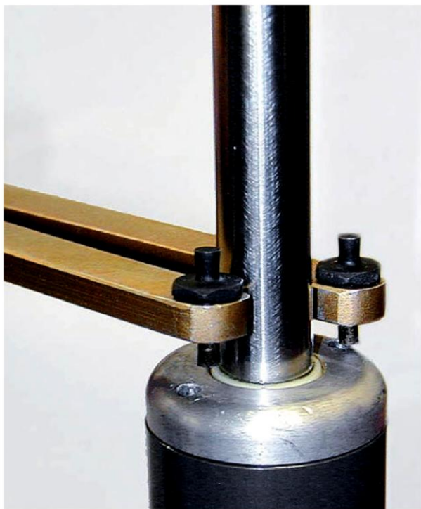
Pin Spanners have a unique design with a reverse taper on the hardened pins. This helps them dig in so that they don’t pop out during use.
