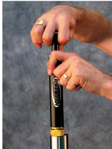
If you are using an Emulator, install it before setting the oil level. Collapse the fork all the way and suck out the excess oil.
