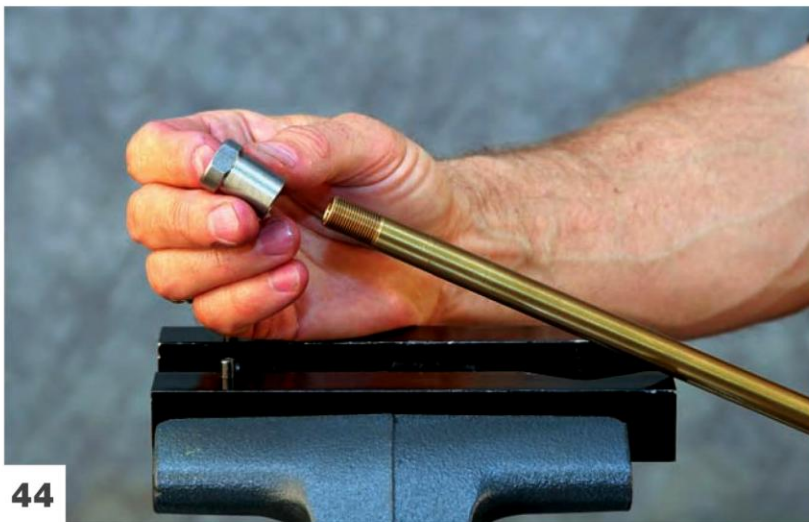
Continue disassembling the cartridge. Remove the damping rod jam nut.
