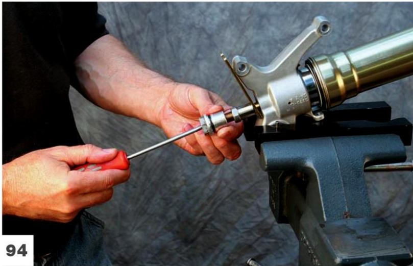
Screw on the rebound adjuster bolt. Use a screwdriver to hold the adjuster screw in position while turning the adjuster bolt. This protects the D-shape rod as we did during disassembly.
