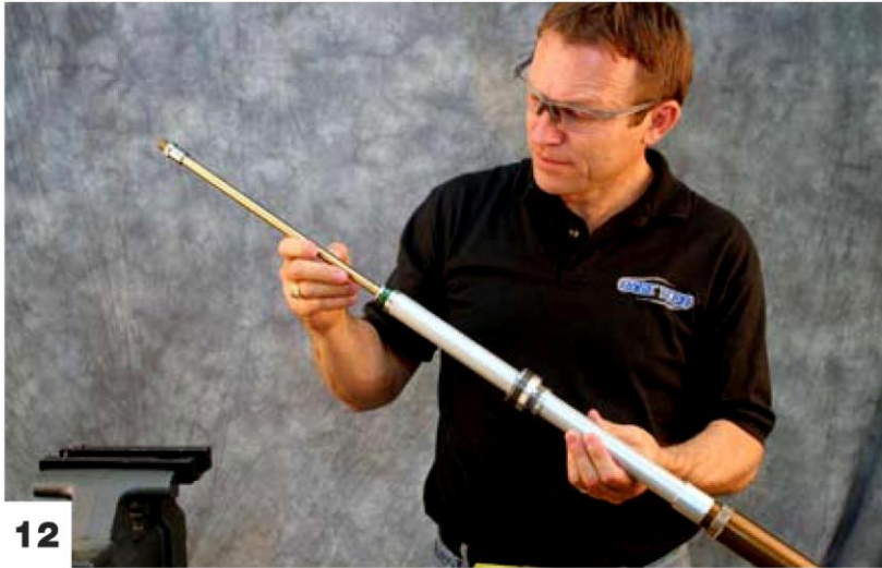
Inspect the cartridge for damage such as dents, wear, etc.
