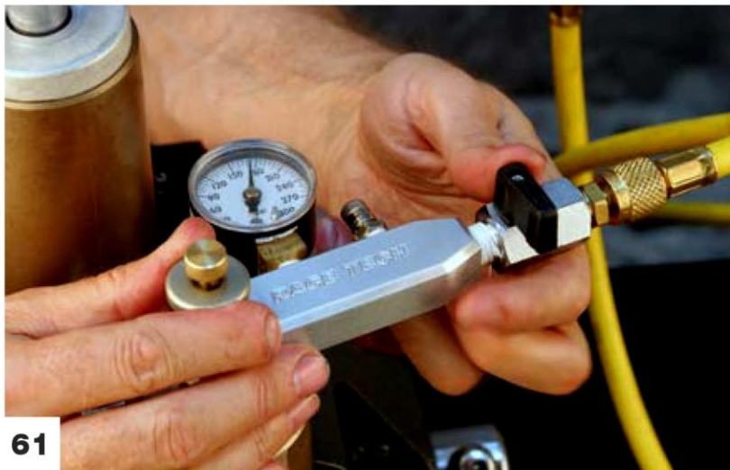
Bleed the shock to the proper pressure.
