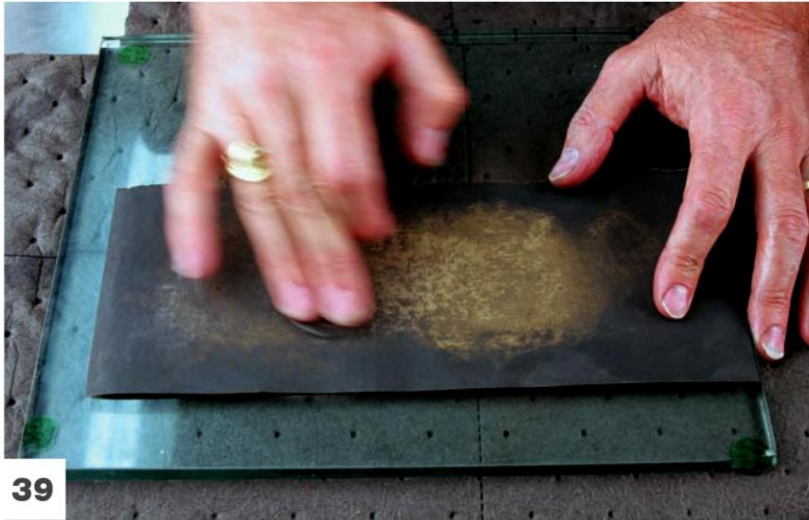
Surface the rebound top plate and install it on the shaft.
