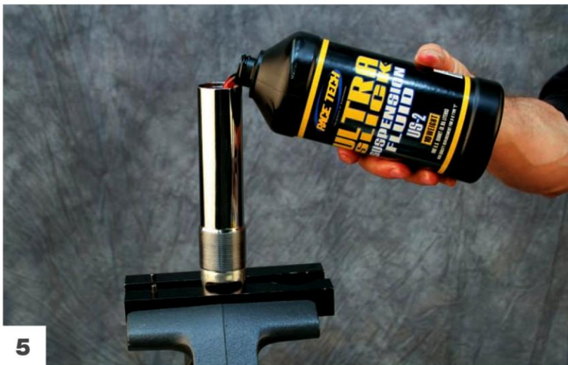
Clean everything, replace seals if needed, and refill the shock body with oil.
