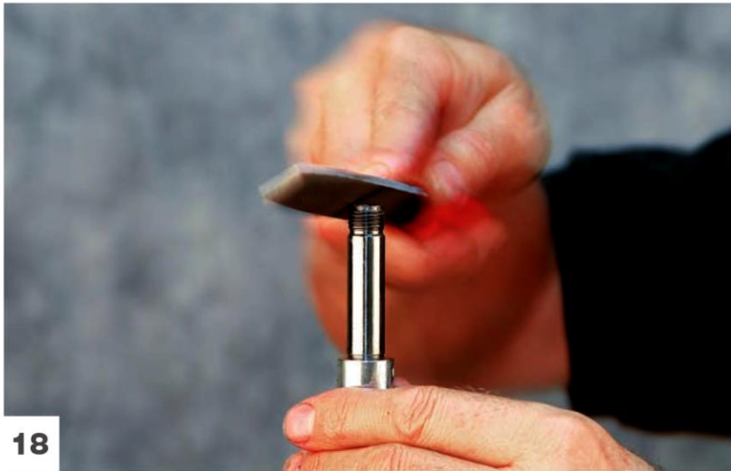
Chamfer the end of the shock shaft.
