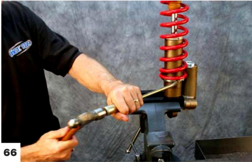
Tighten the lock ring with the shock preload adjuster tool. Grease the preload collar thread before installing the spring.
