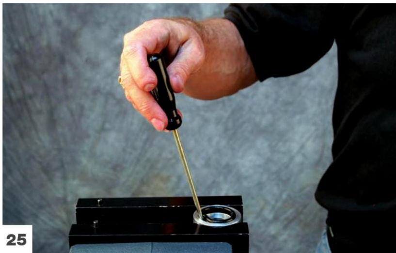
Remove the top-out bumper with a clip tool.
