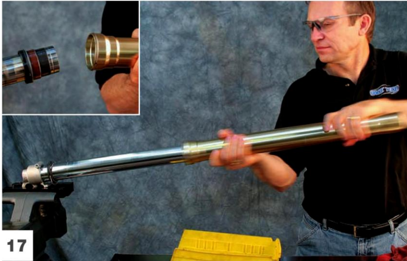
Slide hammer the fork seal and bushings out forcefully.
