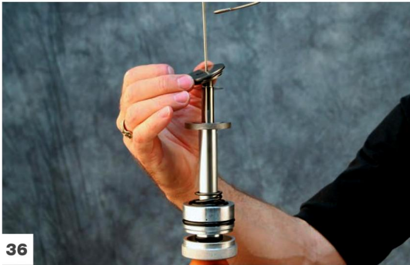
Install the compression valving stack.
