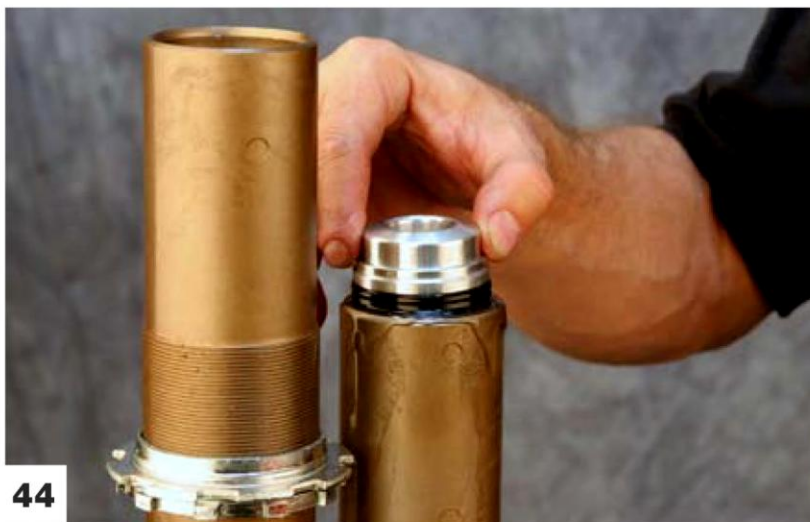
Make sure there is enough oil so that when the bladder goes into the reservoir it overflows.
