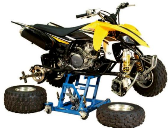
This hydraulic lift is a bit quicker and more stable than the scissor jack shown, but it takes up a little more floor space.
